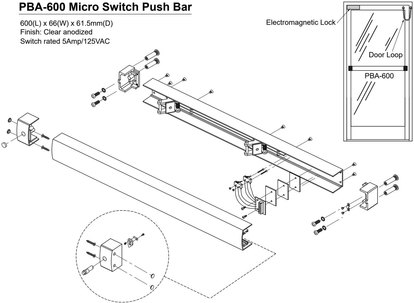
The PBA-600 mechanical micro switch push bar is designed for use on emergency exit doors or large-scale outswing doors. Pressing on the bar activates the interior micro switch, which will remove power to the electromagnetic lock, in turn unlocking the door for immediate egress.
