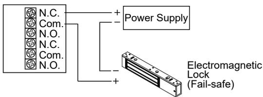
Directly Control the fail-safe electromagnetic lock
