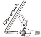
Use a wrench or vice-grip to tightly hold the nut. Then use the included Allen wrench to slowly tighten the screw until it does not turn any further.
