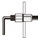
This compresses the blind nut so that it remains permanently fixed in the hole.
