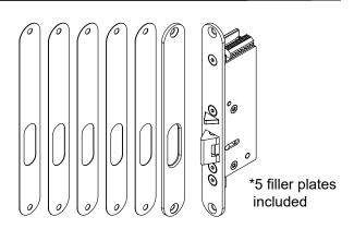
When door is closed and locked, the door gap needs to be less than 5 mm so the auxiliary deadlatch is properly depressed. Add filler plates to compensate for wide door gaps.
