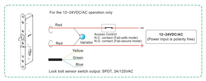
**NOTE:** The varistor (or diode) must be connected across the terminals as shown above. This protects the electromechanical lock from spikes and surges.
