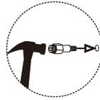
Drill a 9.4mm hole and hammer the blind nut assembly into the hole.
