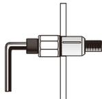
This compresses the blind nut so that it remains permanently fixed in the hole.
