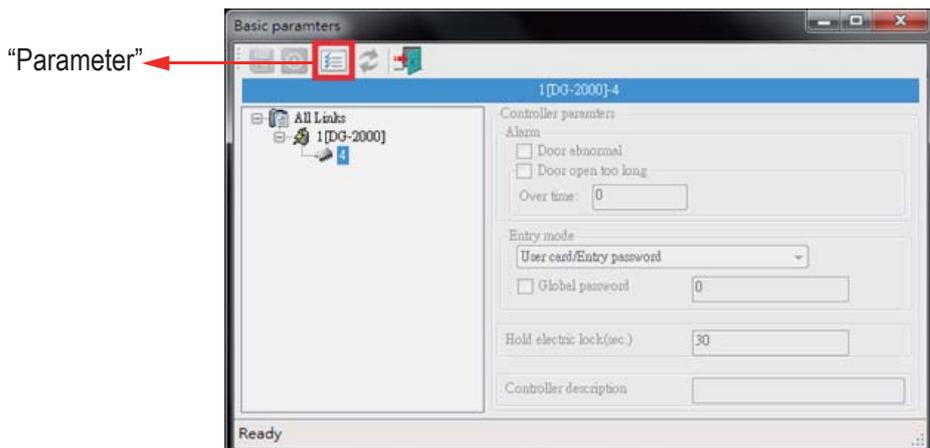
6. Users can enable alarm functions. The timeout for converting door ajar to alarm means if the door still opens for the timeout period after electrified lock release time, the controller will output alarm signal. In the following picture, if the door opens for  $10+15=25$  seconds, the controller will output alarm.
