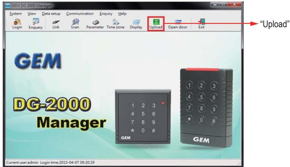
2. Click "Upload" button to retrieve records. After retrieving the records, GEM DG 2000 Manager System can be used to generate reports on records.
