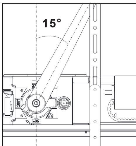
The first arm and pivot post should be kept at a 15 degrees angle (approximately) according to the illustrated door handing when installing the first arm to the operator body. Assemble the first, second and third arm.
