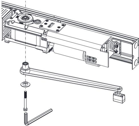
11-4 Open the door such that the arm is at 90 degrees and check the leveling per shown below and adjust leveling accordingly.
