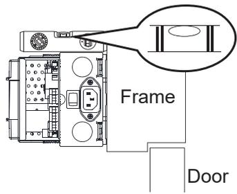
If the operator body obviously slants to the right. Loosen the reducer and adjust the levelness on the right side. In the same way. If the operator body obviously slants to the left. Loosen the reducer and adjust the levelness on the left side.
