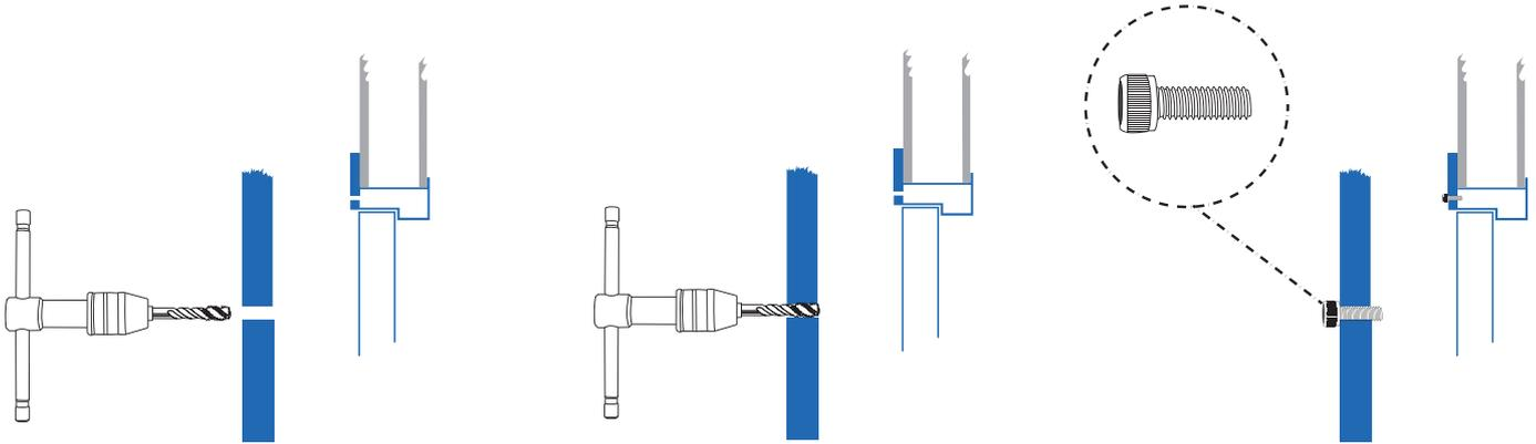
If installing on thin wood or partition boards, a thicker metal plate needs to be added to enhance the sturdiness of the installation site.
