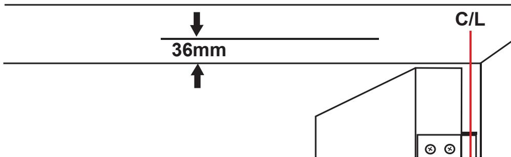
Directions: Check the door hinge centerline, and the two reference lines that are 36 mm away from the bottom line of the header frame.
