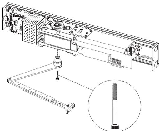
10-1 Turn off power before installing the arm assembly.
