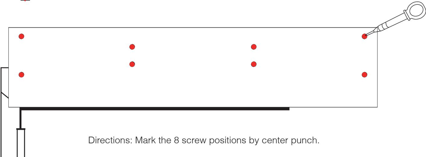
Directions: Mark the 8 screw positions by center punch.
