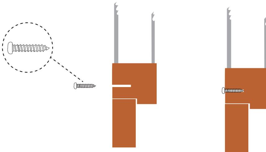
For solid wood frames. Drill 4 mm holes first. Fix Phillips screws.
