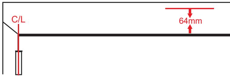
Directions: Check the door hinge centerline, and the two reference lines that are 64 mm away from the bottom line of the header frame.
