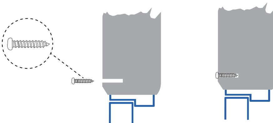
Drill with 5 mm masonry drill bit.
