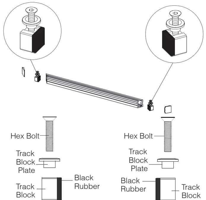
11-7 Use the track block to adjust the opening angle if necessary.
