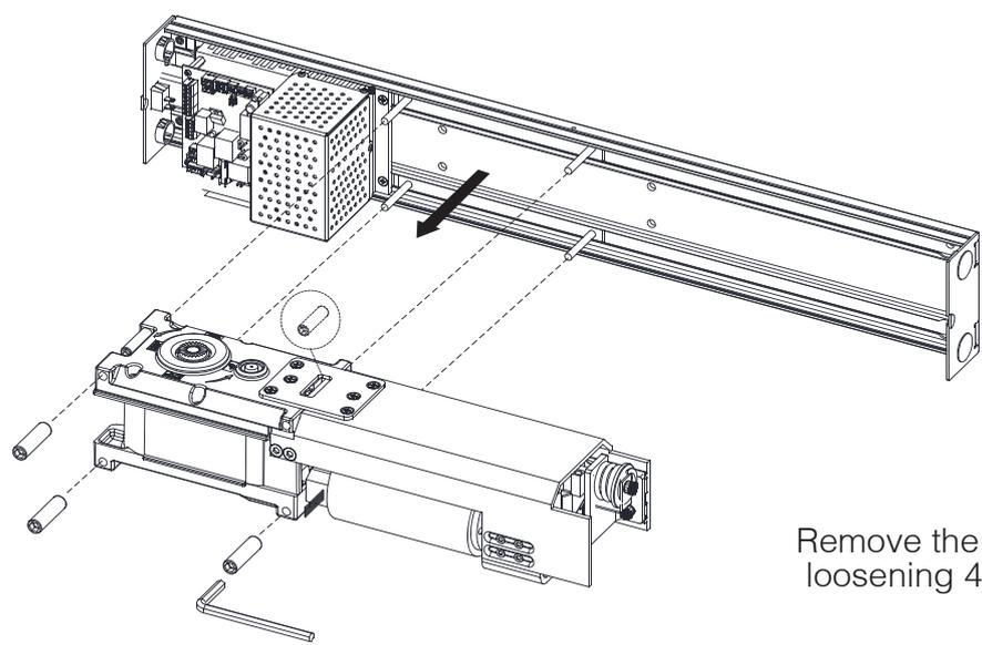
Remove the reducer by loosening 4 screws.
