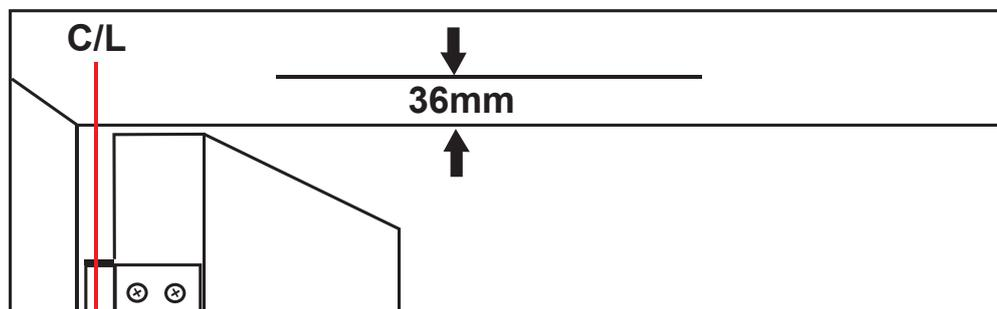
Directions: Check the door hinge centerline, and the two reference lines that are 36 mm away from the bottom line of the header frame.
