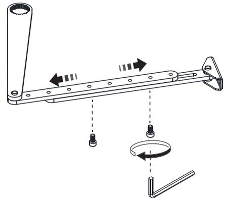
Note: adjust second and third arm according to the door depth. Keep the third arm at right angle to the door leaf.
