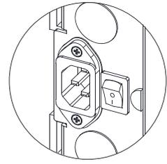
Turn on the power switch on operator. Press the exit button on the operation controller to test the motor operation.
