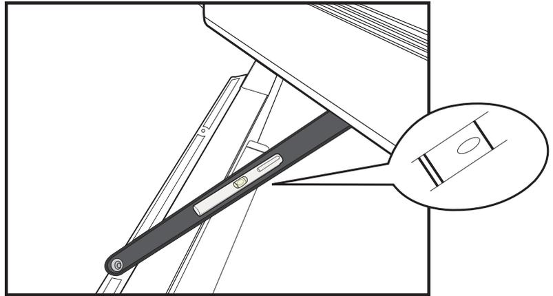
11-5 Assemble the track assembly and sliding arm.
