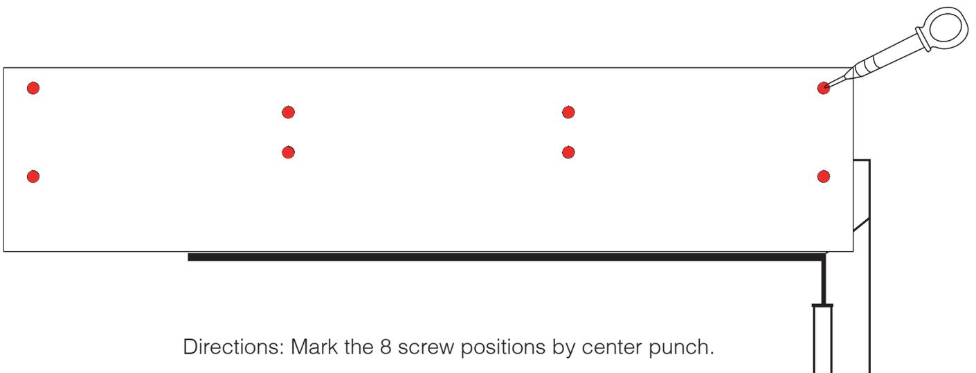
Directions: Mark the 8 screw positions by center punch.
