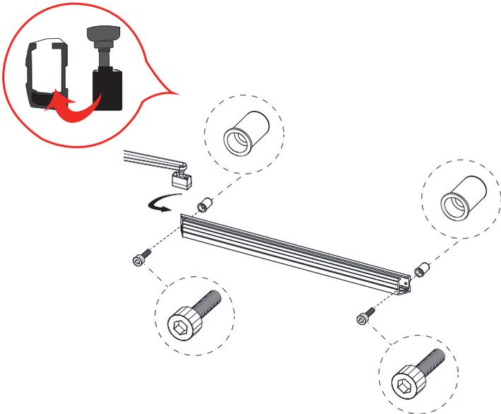
11-6 Put the track block into the track assembly. Place the block with the black rubber side facing the track assembly. The track block installation is up and down rever
