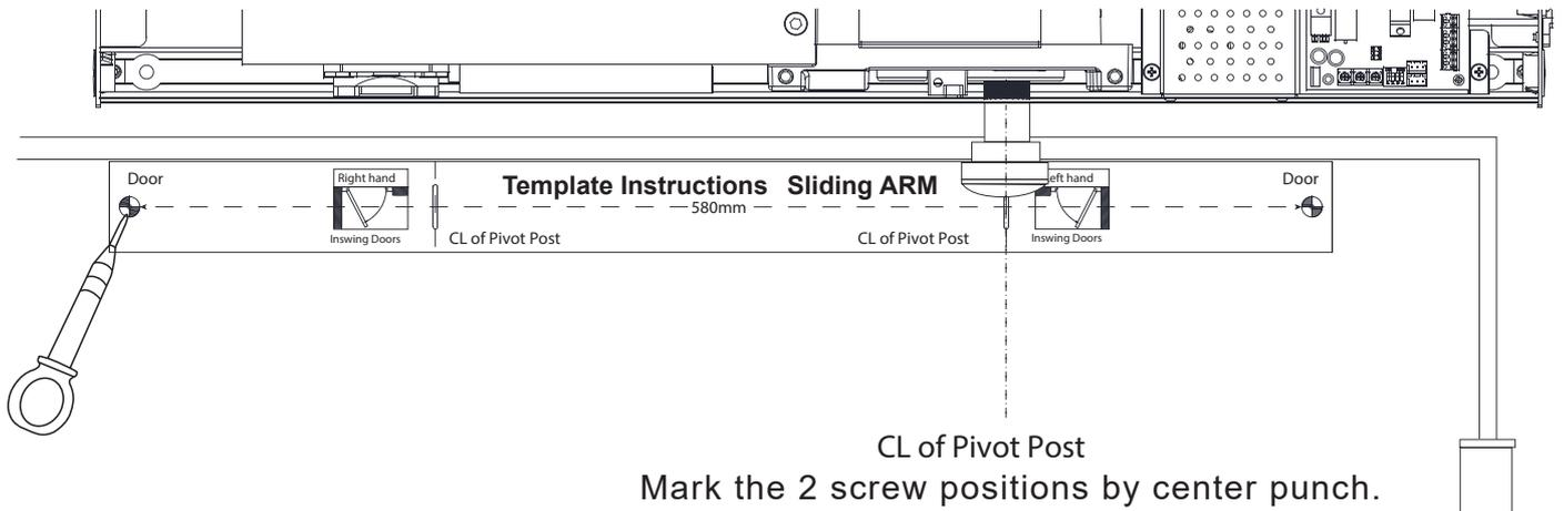
11-3 Fasten the arm to the operator body using the pivot post.
