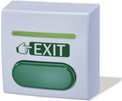
The BlueSwitch PBT-1000BT is ideal for request-to-exit applications to release electromagnetic locks or electric strikes in conjunction with Bluetooth access control systems. Designed with aesthetic appearance for a variety of applications. It operates with 12 to 24 VDC and is enclosed on robust plastic housing.
