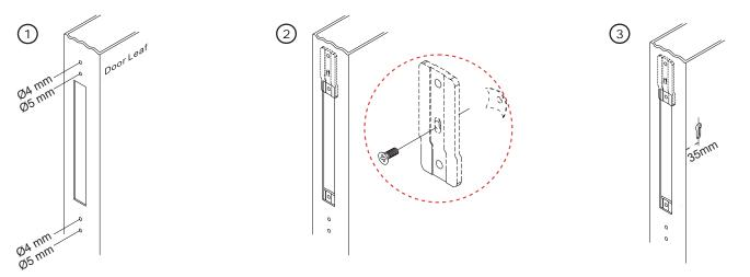
Drill holes and mortise door edge according to the template
