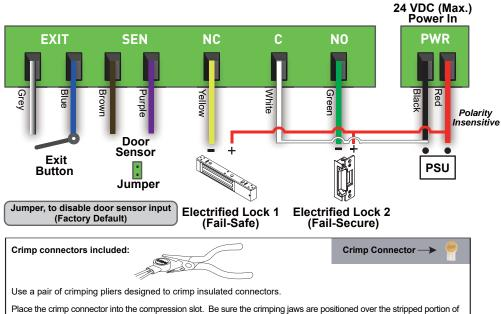
the wire. Squeeze the handles together with enough force to crush the end of the butt splice.
