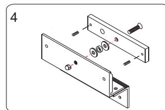
4 Fasten the armature plate to Z Bracket. Insert the rubber washer between them.
