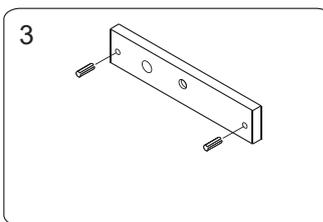
3 Insert the guide pins into the armature plate.
