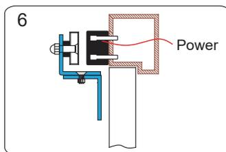
6 Turn on the power of EM-Lock, and let the armature plate bonds to the EM-lock. Adjust the position between the Z bracket and the door frame.
