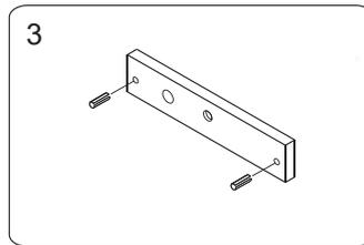
3 Insert the guide pins into the armature plate.
