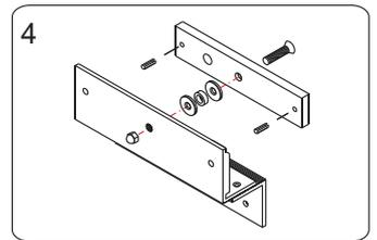
4 Put one rubber washer between armature plate and the Z bracket.
