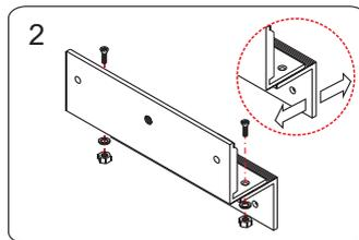
2 Assemble Z bracket. Make sure it is still loose.
