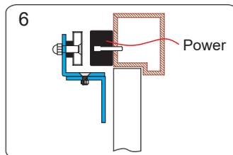
6 Let the armature plate and electromagnet bond together.
