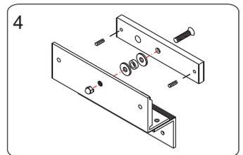
4 Fasten the armature plate to Z bracket. Insert the rubber washer between them.
