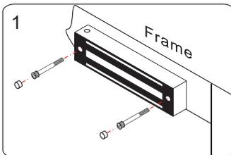
1 Install the electromagnet on the door frame. Make sure the door may be opened / closed.
