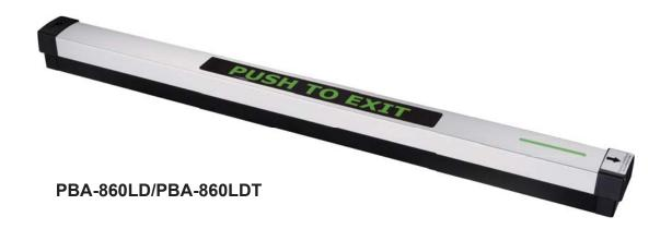
The PBA Micro Switch Bar Series are non-latching push bars designed for use in combination with electric locks for door release. PBA-600LD and PBA-860LD features a LED indicator which allows people to locate the bar in the dark quickly and easily. PBA-600LDT and PBA-860LDT features time delay of up to 50 seconds as well as a volume adjustable buzzer.
