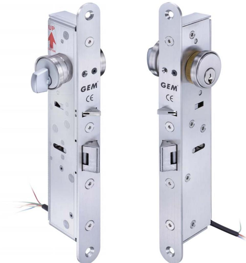
The ML-855M electric lock is a high performance lock designed for single action swing doors. Featuring a double action latchbolt and left/right side adjustable deadlatch tip, the ML-855M allows deadlocking automatically when the door is closed to be secured for ease of use and convenience. The ML-855M can be controlled by card readers/keypads and connected to automatic swing door operators for an integrated access control solution.
