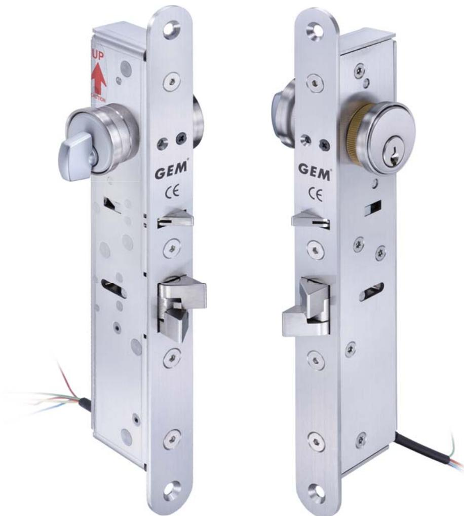
The ML-805M electric lock is a high performance lock designed for single action swing doors. Featuring a double action latchbolt and left/right side adjustable deadlatch tip, the ML-805M allows deadlocking automatically when the door is closed to be secured for ease of use and convenience. The ML-805M can be controlled by card readers/keypads and connected to automatic swing door operators for an integrated access control solution.
