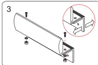
3 Assemble Z bracket. Make sure it is still loose.
