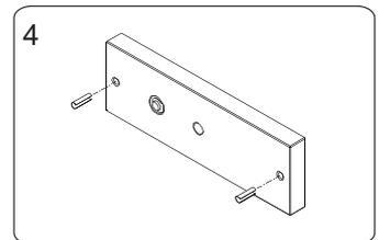
4 Insert the guide pins into the armature plate.
