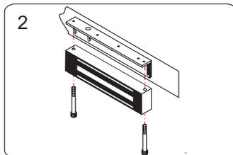
2 Fasten the electromagnet to L bracket with fixing screws.
