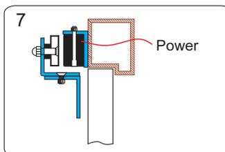
7 Let the armature plate and electromagnet bond together. Press Z bracket to the door leaf.
