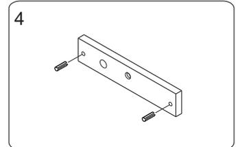
4 Insert the guide pins into the armature plate.
