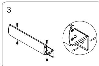
3 Assemble Z bracket. Make sure it is still adjustable.
