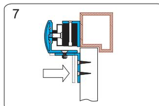
7 Let the armature plate and electromagnet bond together. Press Z bracket the door leaf.
