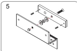
5 Assemble the armature plate and the Z bracket. (Must add rubber washer)
