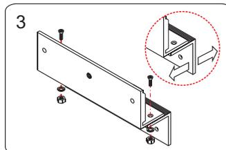
3 Assure that the Z bracket is adjustable. Assemble the Z bracket, and make
