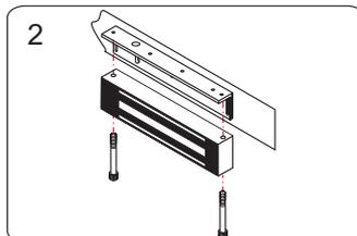
2 Use the fixing bolt to tighten the electromagnet lock on the L bracket
