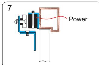
7 Test the tightness and adjust the Z bracket to fit the door.
