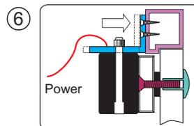
6 Fasten L bracket on the door frame.
