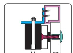
6 Test the unit. Tap the plugs into the electromagnet
