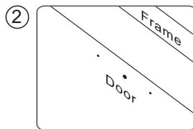
2 Drill the holes marked on the template.
