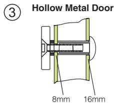
3 Drill a hole 8 mm in diameter through the door. Enlarge the hole to 16 mm from outside.
