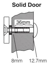
3 Drill a hole 8mm in diameter through the door. Enlarge the hole to 12.7mm from outside. The thickness of the door is 36mm.
