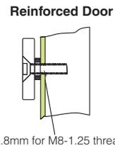
3 Drill a hole 6.8mm in diameter from inside. Screw with a M8-1.25 thread.
