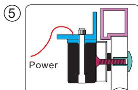
5 Turn on the power of electromagnet. Let the electromagnet and the armature plate bond together. Press L bracket against the door frame.
