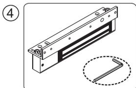
4 Assemble the electromagnet and L bracket with an Allen wrench.
