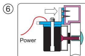
6 Fasten L bracket on the door frame.
