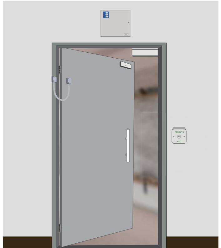
The PBT-090-2WP weather-resistant exit button is designed with an SUS304 stainless steel box for surface mount installation in indoor and light weathering outdoor settings. The exit button itself is a 19mm stainless steel button with IP54 sealing and can operate in temperature ranging from -20°C to 70°C.
