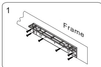
1 Install L bracket on the door frame. Make sure the door may be opened / closed.
