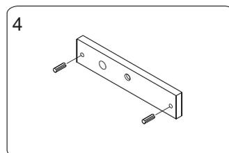
4 Insert the guide pins into the armature plate.
