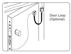
The door loop protects the wiring from damage at the door hinge.
