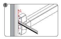
a. Measure the exit device latch position on the door.
