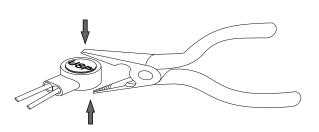
Place the wire inside the connector and use pliers to press down on the head of the connector evenly.
