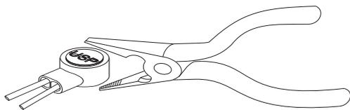
Using crimper or pliers and pressing the header of connector down to even position
