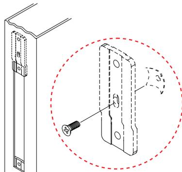
Position screws for fasten Fixing Lugs
