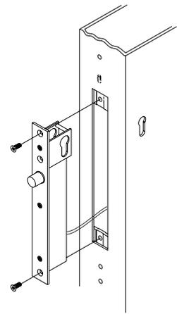
Connect power cable to electric dropbolt
