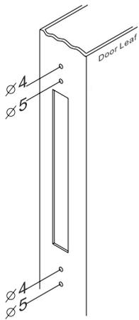
Drill and cut as template indicated for dropbolt
