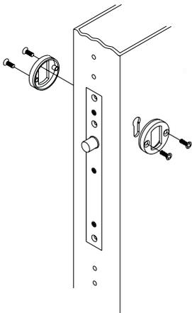
Insert electric dropbolt into position, attach to Fixing Lugs and base
