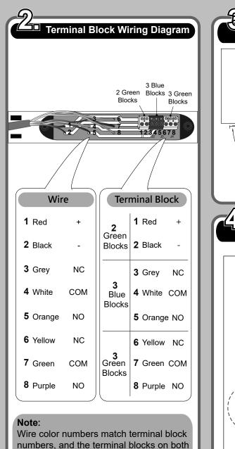
For each side, the Red wire 1 is connected to the terminal 1 of the Green Block, the Black wire 2 is connected to the terminal 2 of the Green Block, and so on.
