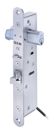
The ML-705M electric lock is a high performance lock designed for single action swing doors. Featuring a double action latchbolt and left/right side adjustable deadlatch tip, the ML-705M allows deadlocking automatically when the door is closed to be secured for ease of use and convenience. The ML-705M can be controlled by card readers/keypads and connected to automatic swing door operators for an integraed access control solution.
