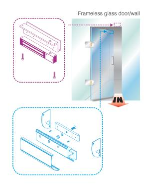
MG-300LZ Brackets are designed for EM-150 Electromagnetic Lock to be installed on full frameless glass doors. The lock and the armature plate are wrapped up by the brackets to make the lock aesthetically appealing.
