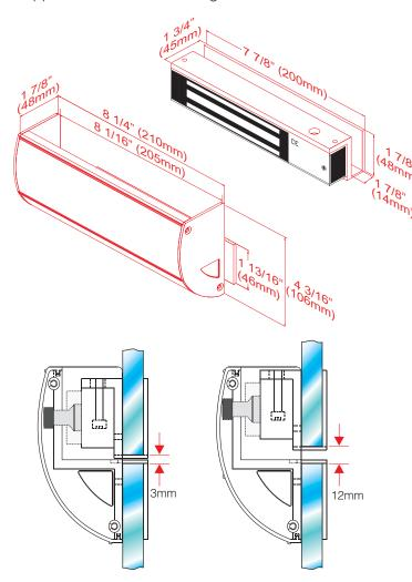
The thickness of glass should be 10~13 mm and the position of armature plate and electromagnet can be adjusted depending on the door gap ranging from 3 mm to 12 mm.
