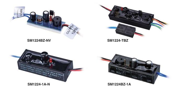
The SM Series in-line security rectifiers can serve as an added security to your access control system. They have a built-in rectifier component and are able to receive input voltages from 12 to 24V AC or DC and provide constant 12 VDC output voltage.
